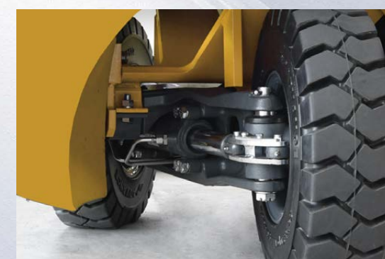
Casting steering bridge
